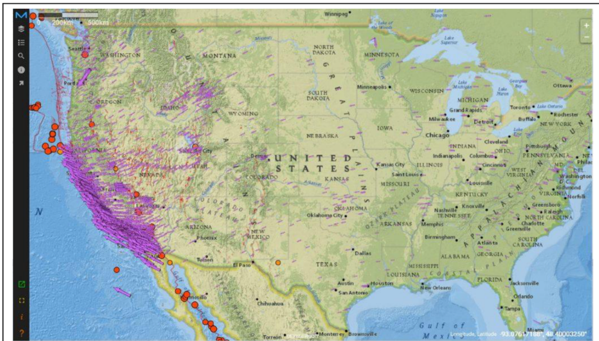
Figure 11: An example of ITRF2004 horizontal velocities estimated from the combined time series of JPL and SIO. Significant ( M > 6 ) earthquakes denoted by red circles. This is a screen shot from MGviz (section 10.2), http://mgviz.ucsd.edu/?mission=ESESES
