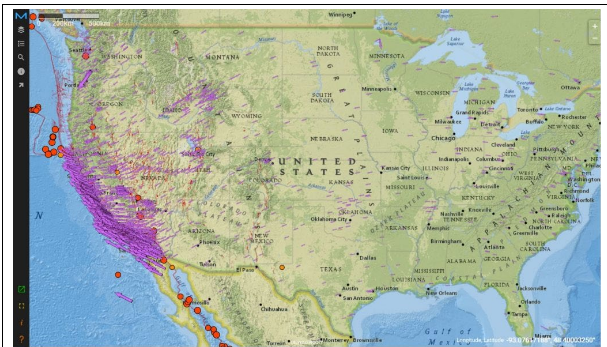
Figure 11: An example of ITRF2004 horizontal velocities estimated from the combined time series of JPL and SIO. Significant ( M > 6 ) earthquakes denoted by red circles. This is a screen shot from MGviz (section 10.2), http://mgviz.ucsd.edu/
